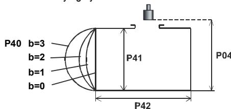
Spherical tank  $a = 4, b = 0$
